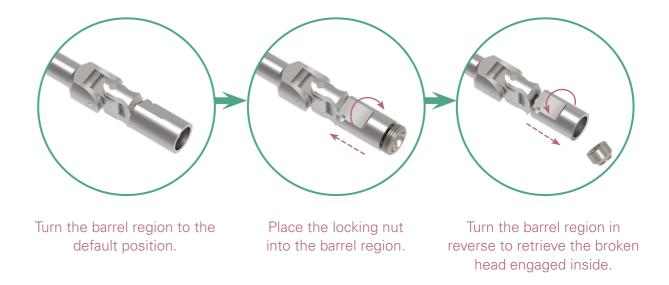
The cap can be retrieved by using the **T20 Universal Screwdriver** when needed.
